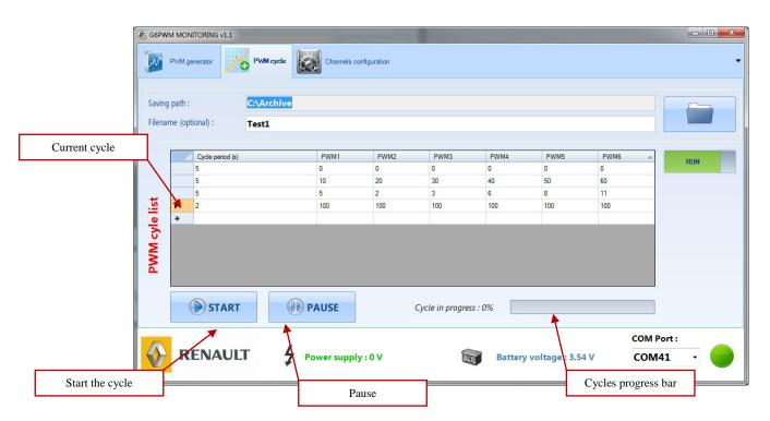
Creating a program is very straightforward. First the time of how long each PWM generation can last (in seconds) has to be set then the PWM values of each channel can filled.
