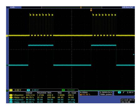
The signal generated by the G6PWM in this example is 50Hz 40% PWM ratio TTL (in blue) and the read back when the level is high is 1KHz 45% PWM ration (in yellow).
